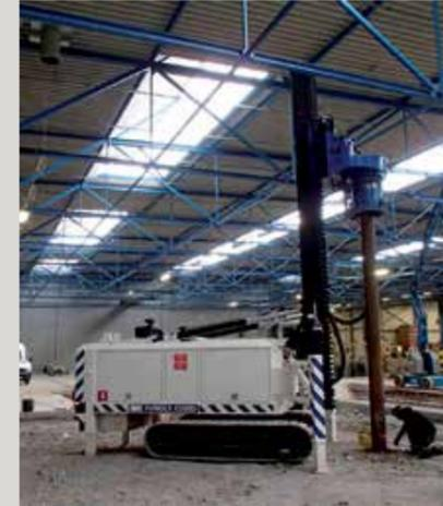
The machine is operated using a remote control device. This gives the machine operator the freedom to move around the machine and obtain an optimal picture of the operations.
