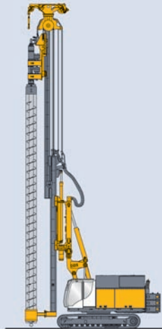
VdW Vor-der Wand Bohren Front-Of-Wall drilling
