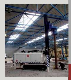
The machine is operated using a remote control device. This gives the machine operator the freedom to move around the machine and obtain an optimal picture of the operations.
