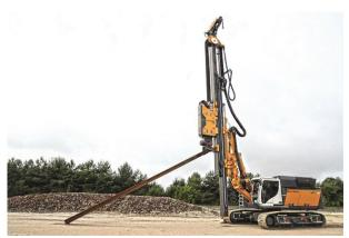
(1) The sheet pile driving assistant is an effective tool for accurate and rapid handling of sheet pile elements.
