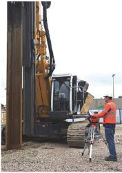
(2) The radio remote control is also used to remotely control the safe assembly and disassembly of the RG rigs.
