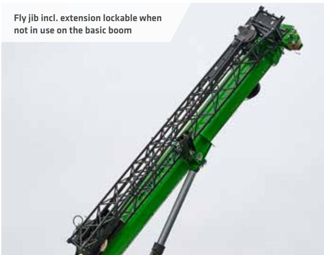
Fly jib incl. extension lockable when not in use on the basic boom
