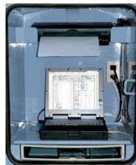
Automatic monitoring of piling conditions by an on-board computer
