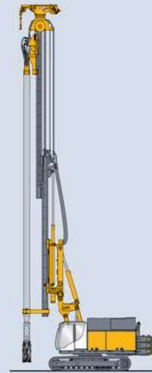
CSM Cutter Soil Mixing
