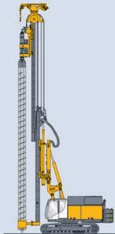
VdW Vor-der Wand Bohren Front-Of-Wall drilling
