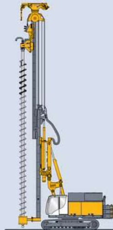
MB Schneckenbohren Auger drilling
