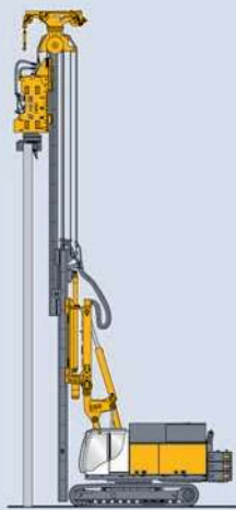
MR Hydraulikrüttler Hydraulic vibrator
