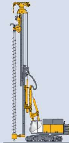
MB Schneckenbohren Auger drilling
