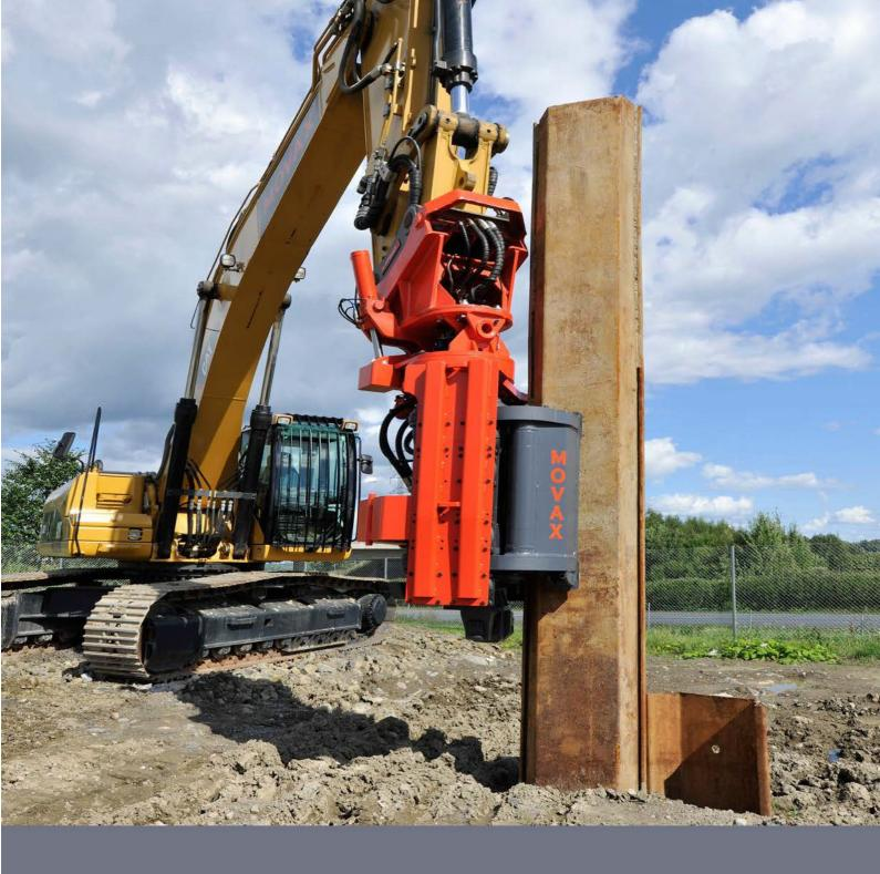
Maximum power: 285.6 HP Operating weight: 36.2 t Max. bucket capacity: 2.01 m<sup>3</sup>
