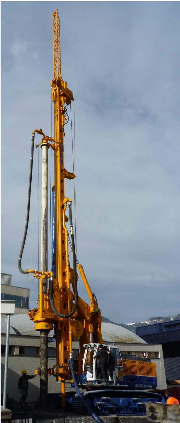
Figure 3: BG with FDP front-end equipment as well as kelly and lattice mast extensions
