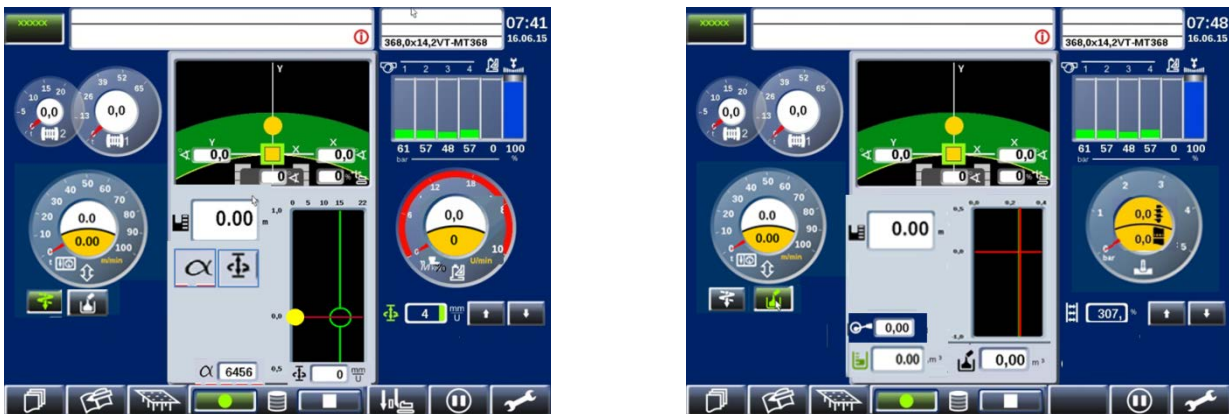
Figure 5: B-Tronic screen – left: 'Drilling Assistant' - right: 'Extraction Assistant'
