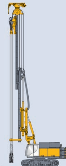
CSM Cutter Soil Mixing
