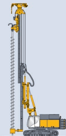
MB Schneckenbohren Auger drilling
