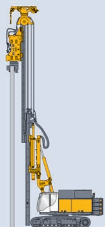
MR Hydraulikrüttler Hydraulic vibrator
