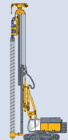
VdW Vor-der Wand Bohren Front-Of-Wall drilling
