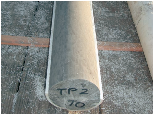
Cut-open inner plastic tube with hardened core
