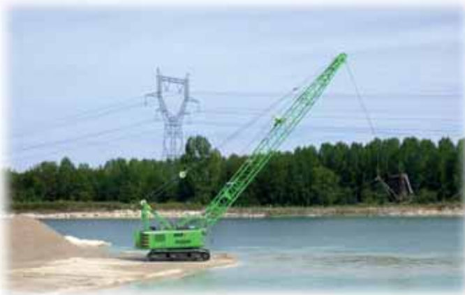
Image 1: Tossing out the empty bucket
