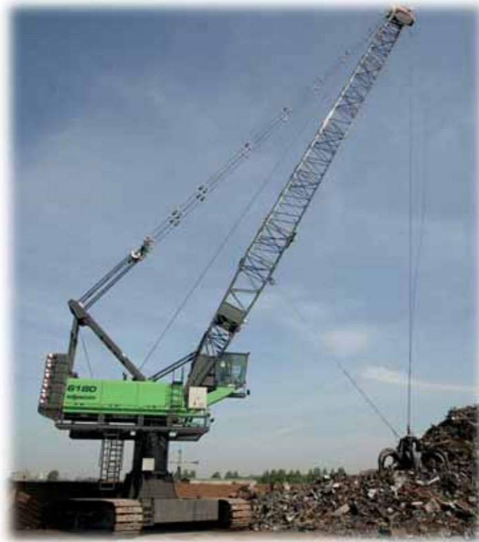
SENNEBOGEN 6180HD with multi-shell grab [source SENNEBOGEN]
