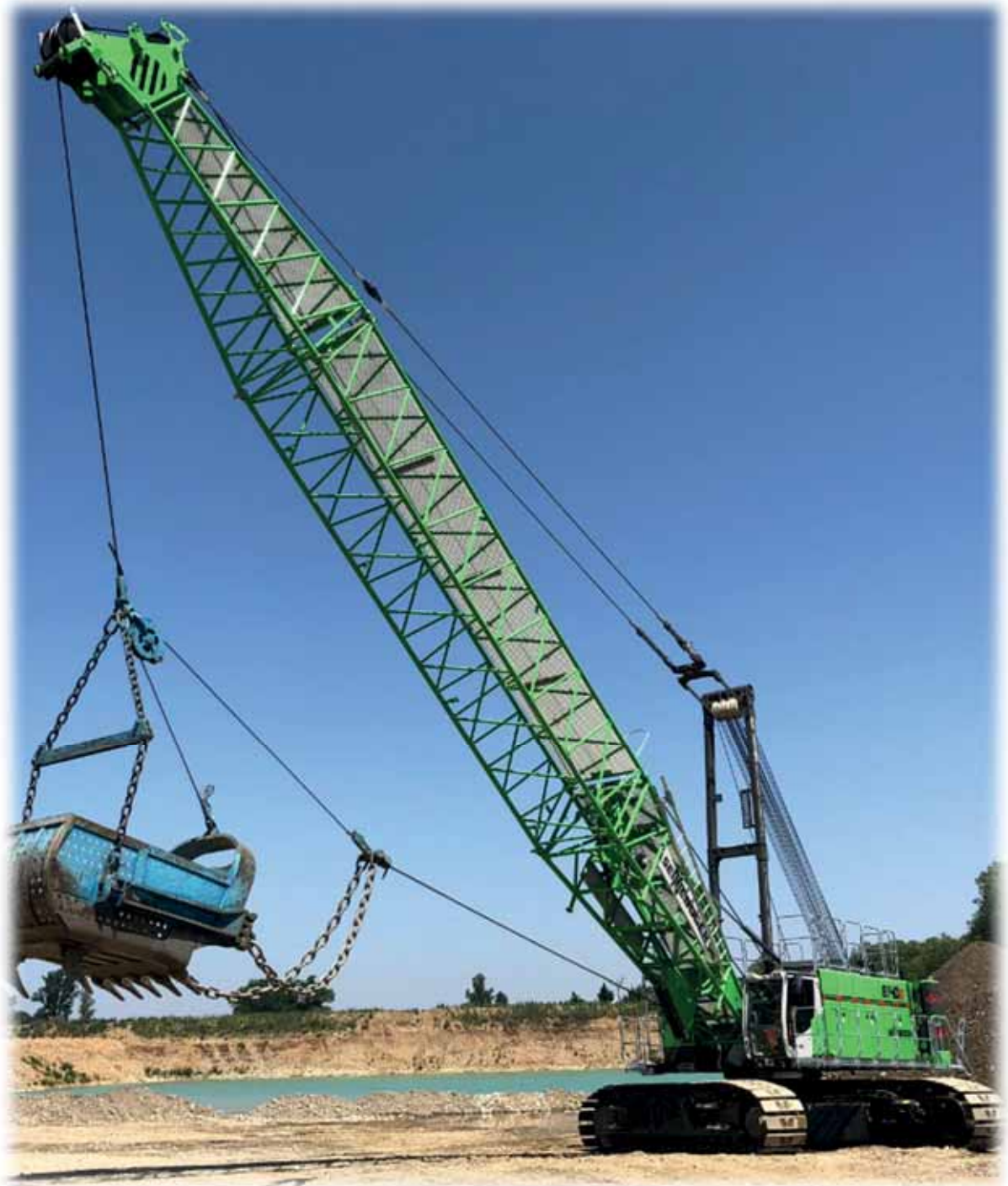
SENNEBOGEN 6140 with dragline bucket [source: SENNEBOGEN]
