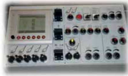
Control panel for control of leader and attachments – SENNEBOGEN 6100XLR [source: SENNEBOGEN]
