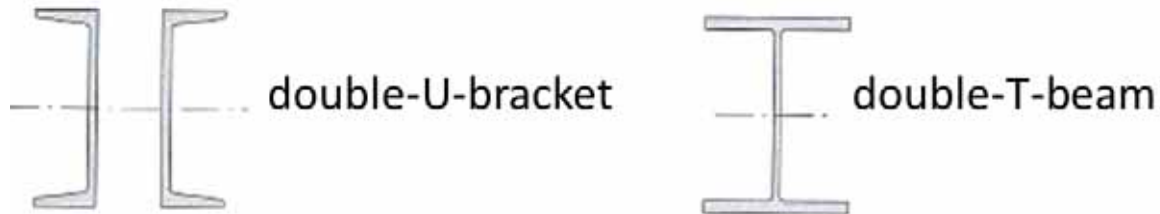
Steel profiles for insertion [source: SENNEBOGEN]
