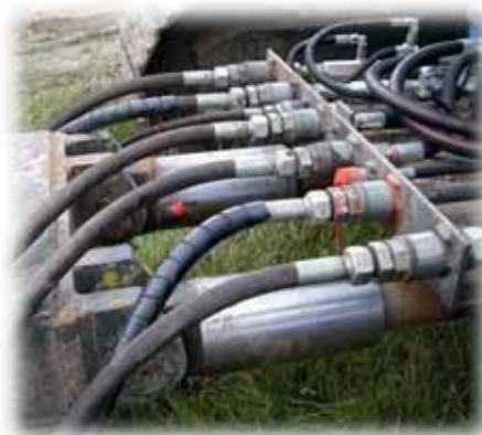
Hydraulic connection – casing oscillator on the middle bridge of the undercarriage SENNEBOGEN 630 HD [Source: SENNEBOGEN]
