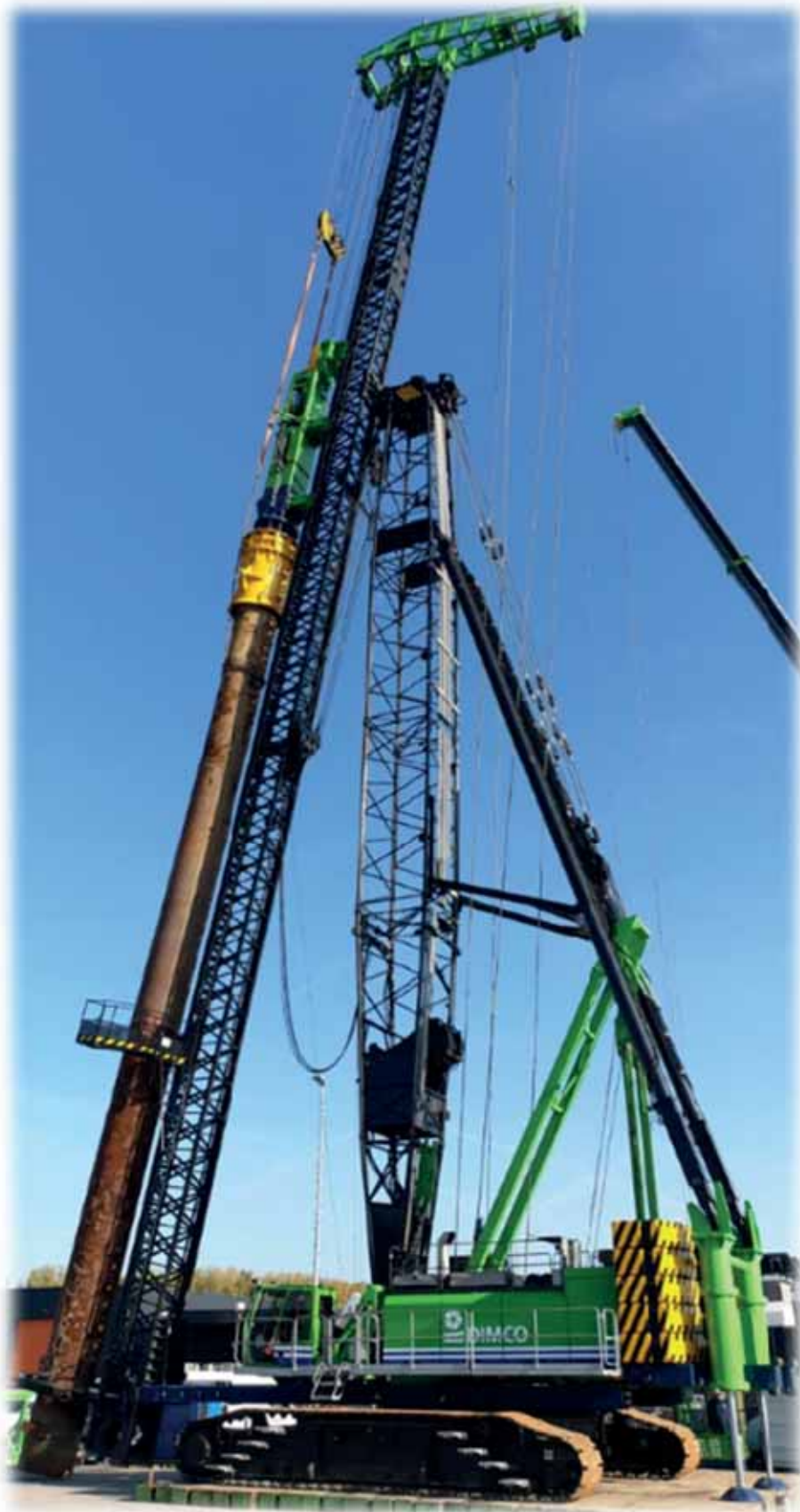
SENNEBOGEN 6180HD with leader system [source: SENNEBOGEN]
