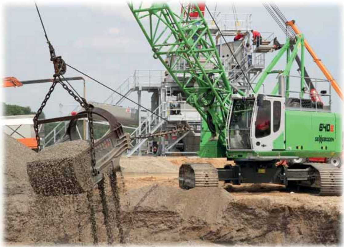
SENNEBOGEN 640HD with 1.7 m 3 dragline bucket – Germany [source SENNEBOGEN]
