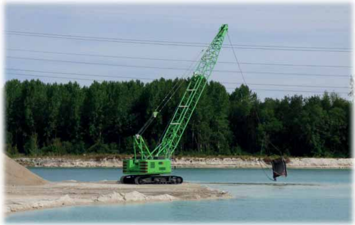
SENNEBOGEN 655HD with dragline bucket – France [source SENNEBOGEN]
