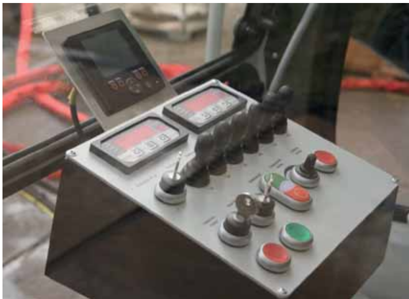
Example of control panel of the leader control system [source: SENNEBOGEN]
