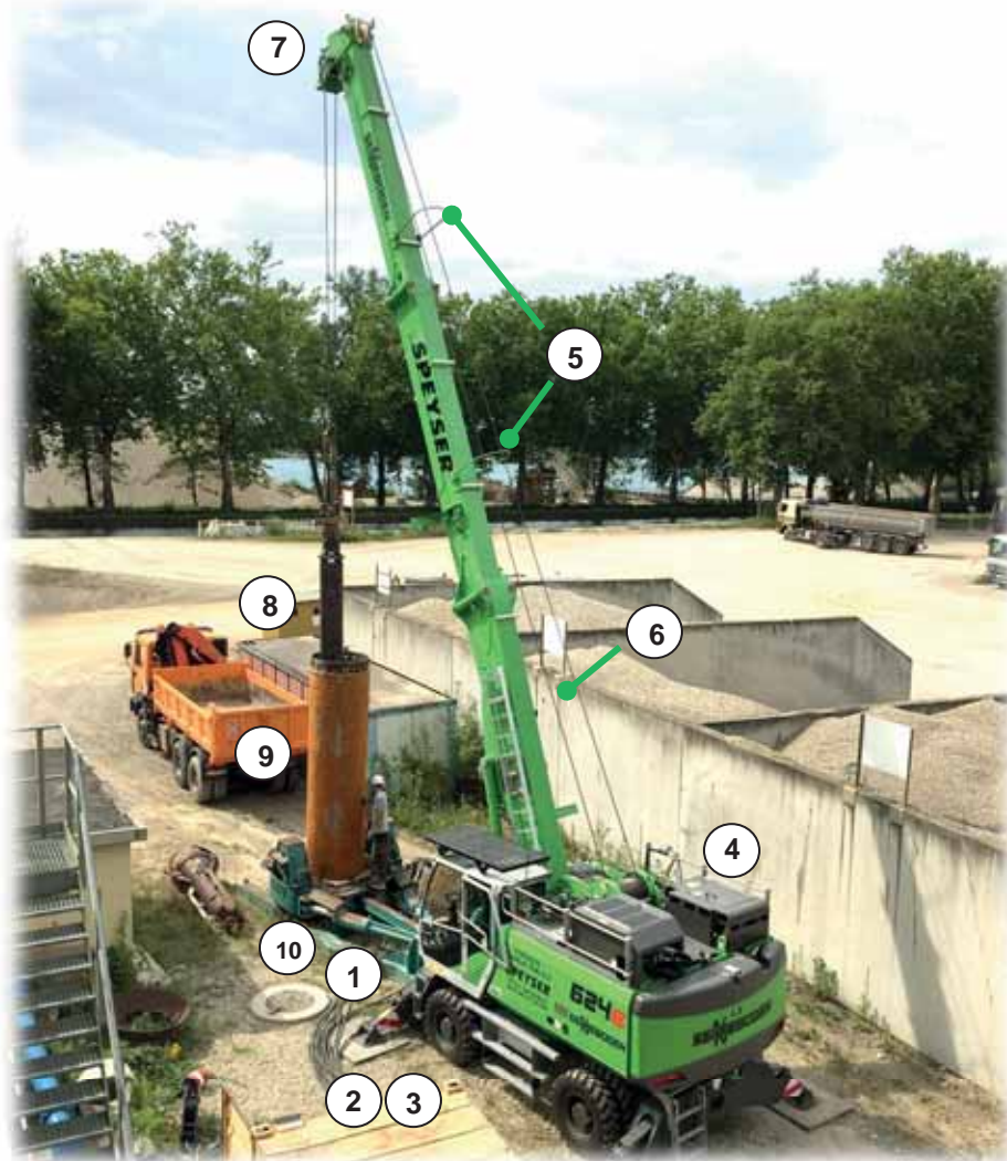
SENNEBOGEN duty cycle crane equipment for pile grab with casing oscillator [source: SENNEBOGEN]
