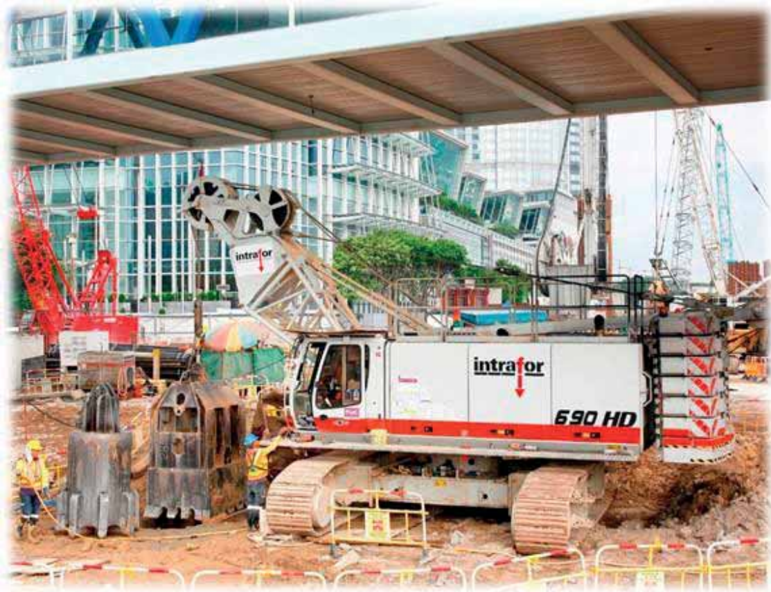
SENNEBOGEN 690 HD with “low head room” boom and boom head [source: SENNEBOGEN]
