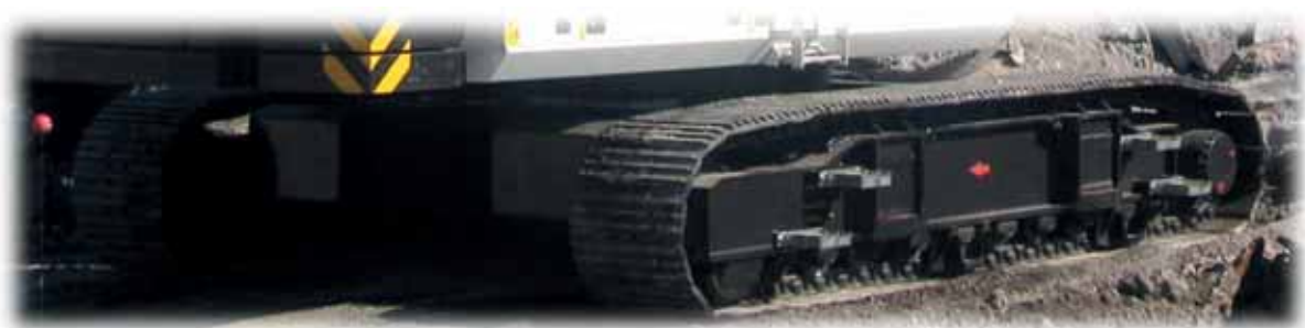
Undercarriage 6100HD drop ball [source: SENNEBOGEN]
