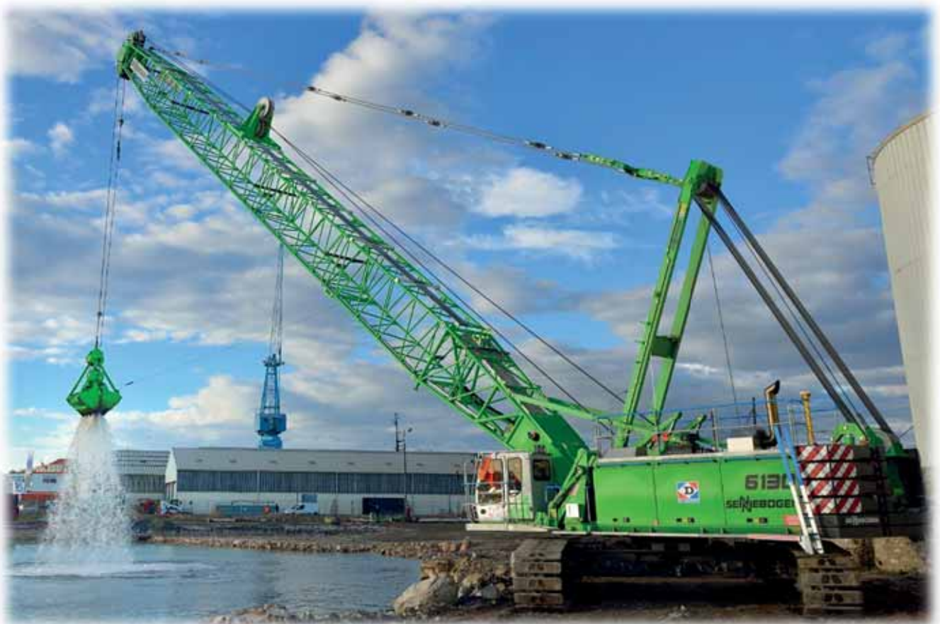
SENNEBOGEN 6130HD with double shell grab [source SENNEBOGEN]
