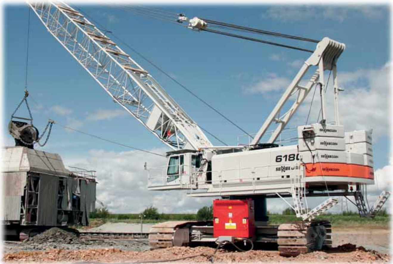
SENNEBOGEN 6180HD electric motor with 6.0 m 3 dragline bucket – Great Britain [source SENNEBOGEN]
