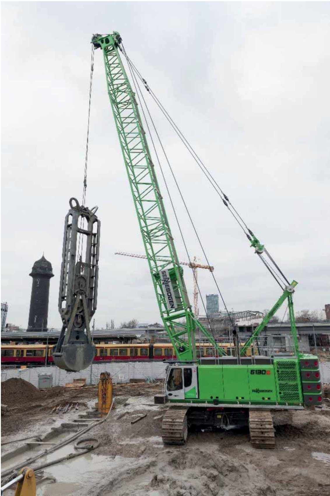
SENNEBOGEN 6130HD with mechanical diaphragm wall grab / Germany [source: SENNEBOGEN]
