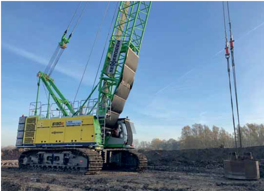
SENNEBOGEN 6130HD with drop plate [source SENNEBOGEN]
