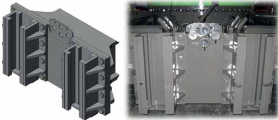
Mechanical connection for casing oscillator – middle bridge of the undercarriage SENNEBOGEN 690HD [source: SENNEBOGEN]
