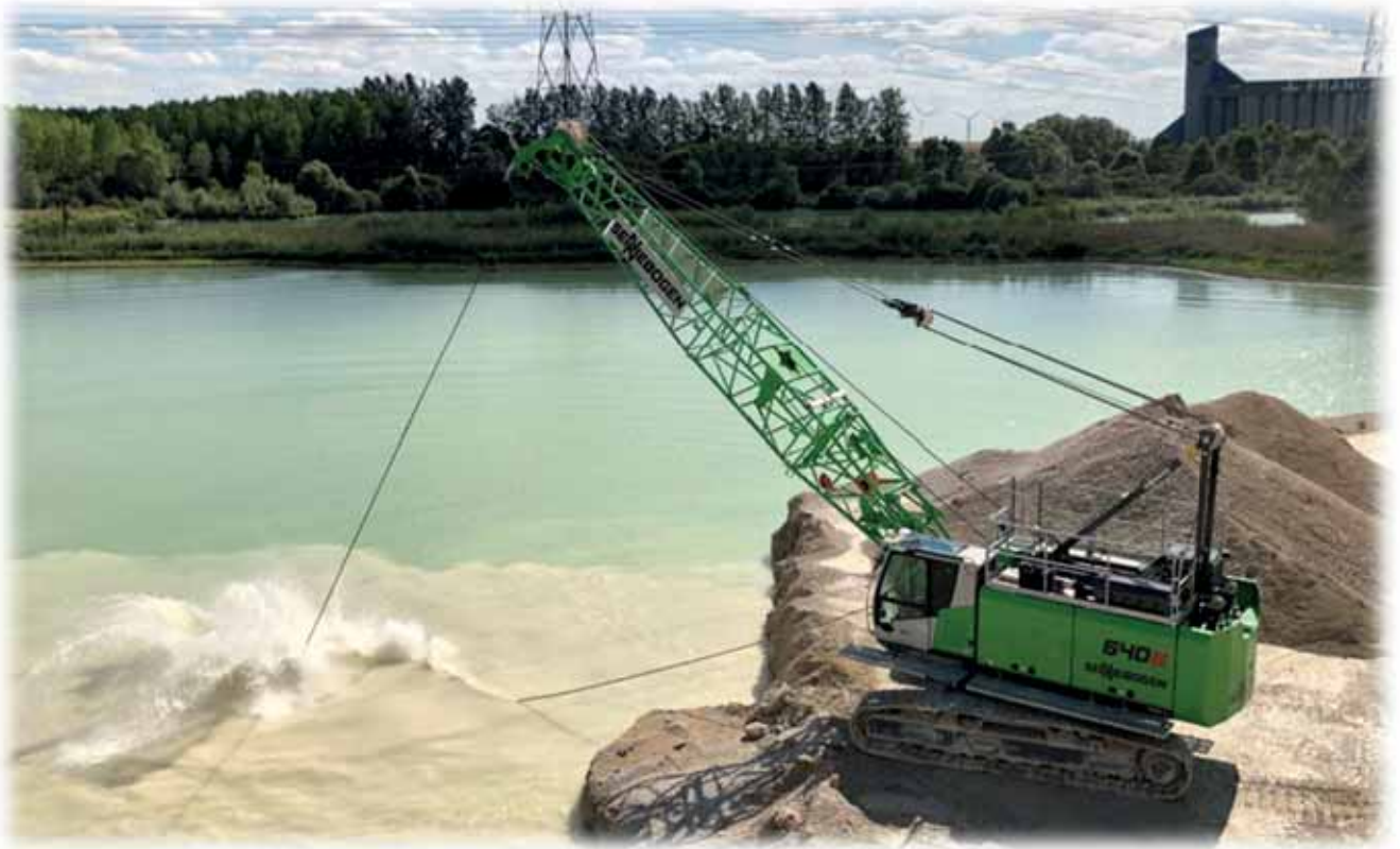
SENNEBOGEN 640HD with dragline bucket – France [source SENNEBOGEN]
