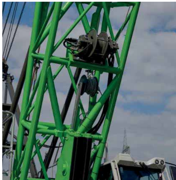
Grab steadying winch 670HD installed in the basic boom section [source: SENNEBOGEN]
