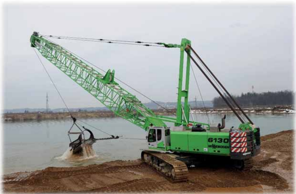
SENNEBOGEN 6130HD with dragline bucket – Austria [source SENNEBOGEN]
