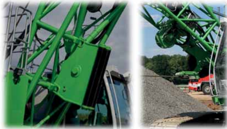
Detail graphic of fairlead [source: SENNEBOGEN]
